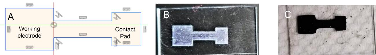
Figure 4. (A) A computer-aided design of a planar electrode for proof-of-concept studies followed by the 3D printed designs before (B) and after pyrolysis (C) supporting that 3D printed designs can be pyrolyzed using the fabrication scheme above.
