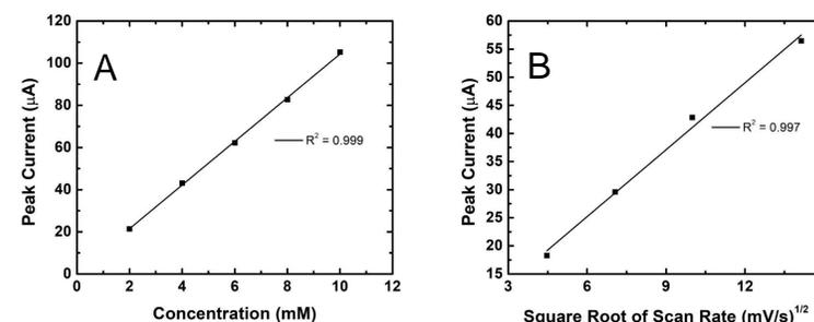
Figure 6. (A) Plot of peak current vs potassium ferricyanide concentration and (B) plot of peak current vs the square root of scan rate for cyclic voltammograms collected with a pyrolyzed 3D printed electrode, Ag/AgCl reference electrode, and Pt counter electrode. 1.0 M potassium nitrate supporting electrolyte was used for all cyclic voltammograms. Each plot demonstrates a linear relationship as predicted by the Randles-Sevcik equation.
