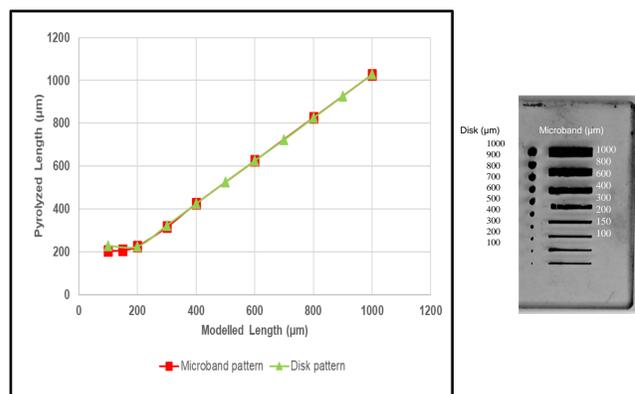
Figure 2. A research grade optical microscope was used to dimensional lengths of disk and microband electrodes pictured to the right. The points were overlaid on a graph to determine a minimum feature size that can be produced with this method. The smallest feature using this method so far is about 200 μm.
