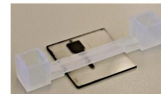
Figure 8: A 55 cm long device with a 0.3 cm x 3 cm channel and two wells. There is also a 26 mm gap in the bottom of the device where the electrode
