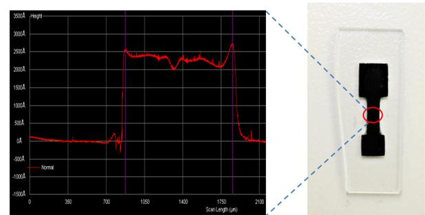
Figure 3. A step height measurement using stylus profilometry was completed on a 3D printed PPE and averaged 250 nm. A silica probe runs across the quartz and when it reaches the PPE it steps up and drags across the device until it steps done to the quartz again.
