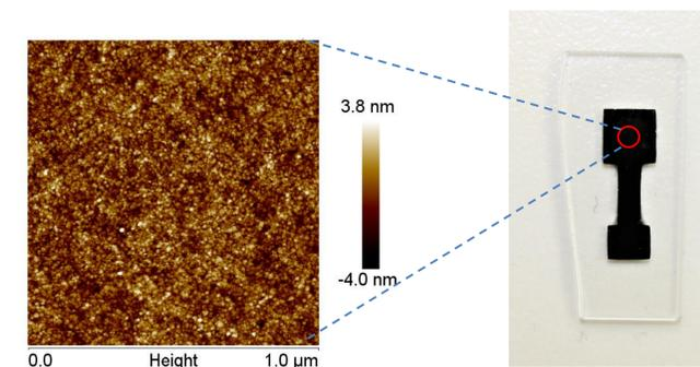
Figure 7. A surface roughness analysis was completed on a PPE device using atomic force microscopy (AFM). A silica probe was swept across a 1 micrometer X 1 micrometer area to determine a surface roughness of 1.8 nm on the device as a preliminary result. This measurement is similar to a commercial glassy carbon electrode.
