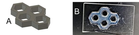
Figure 9. (A) Computer-aided design of a honeycomb electrode structure. (B) 3D printed honeycomb structure.
