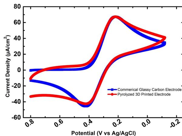
Figure 5. Cyclic voltammograms of a commercial glassy carbon electrode (blue) and a pyrolyzed 3D printed electrode (red) collected in a 4 mM potassium ferricyanide and 1.0 M potassium nitrate solution at a scan rate of 100 mV/sec with a Ag/AgCl reference electrode and Pt counter electrode.
